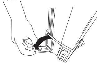
② Place closed unit with carry handle on left side (from audience perspective). Depress two buttons on front and back of housing (clearly marked) with thumb and index finger. Open screen slowly to desired width.
